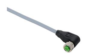
Murrelektronik connection cable, M12 right-angle female to pigtail, 5-pole, PUR jacket, gray, shielded, 16.4ft/5m cable length, IP67.
