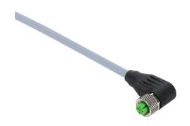
Murrelektronik connection cable, M12 right-angle female to pigtail, 4-pole, PUR jacket, gray, shielded, 32.8ft/10m cable length, IP67.
