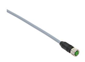
Murrelektronik connection cable, M12 axial female to pigtail, 5-pole, PUR jacket, gray, shielded, 32.8ft/10m cable length, IP67.
