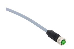
Murrelektronik connection cable, M12 axial female to pigtail, 5-pole, PUR jacket, gray, shielded, 16.4ft/5m cable length, IP67.
