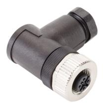
Murrelektronik connector, field-wireable, M12 nut 5-pin female right-angle connection, accepts cable diameter size 6-8mm, 18 AWG, screw terminal connection, IP67.
