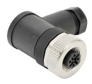
Murrelektronik connector, field-wireable, M12 nut 4-pin female right-angle connection, accepts cable diameter size 4-6mm, 18 AWG, screw terminal connection, IP67.
