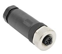
Murrelektronik connector, field-wireable, M12 nut 5-pin female axial connection, accepts cable diameter size 6-8mm, 18 AWG, screw terminal connection, IP67.
