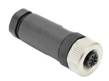
Murrelektronik connector, field-wireable, M12 nut 4-pin female axial connection, accepts cable diameter size 6-8mm, 18 AWG, screw terminal connection, IP67.
