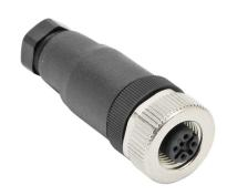
Murrelektronik connector, field-wireable, M12 nut 5-pin female axial connection, accepts cable diameter size 4-6mm, 18 AWG, screw terminal connection, IP67.
