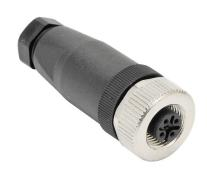
Murrelektronik connector, field-wireable, M12 nut 4-pin female axial connection, accepts cable diameter size 4-6mm, 18 AWG, screw terminal connection, IP67.
