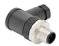
Murrelektronik field wireable connector, M12 barrel 4-pin male right-angle connection, accepts cable diameter size 4-6mm, 18 AWG, screw terminal connection, IP67.
