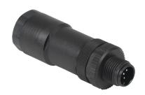
Murrelektronik connector, field-wireable, 5-pin M12 axial male A-coded, accepts cable diameter size (2) 1-3mm or (2) 4-5mm, 18 AWG, screw terminal connection, IP67.
