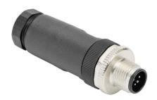
Murrelektronik field wireable connector, M12 barrel 5-pin male axial connection, accepts cable diameter size 6-8mm, 18 AWG, screw terminal connection, IP67.
