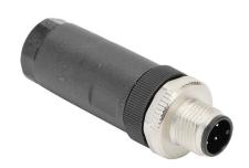
Murrelektronik connector, field-wireable, M12 barrel 4-pin male axial connection, accepts cable diameter size 6-8mm, 18 AWG, screw terminal connection, IP67.
