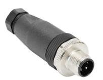
Murrelektronik connector, field-wireable, M12 barrel 5-pin male axial connection, accepts cable diameter size 4-6mm, 18 AWG, screw terminal connection, IP67.
