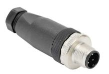
Murrelektronik connector, field-wireable, M12 barrel 4-pin male axial connection, accepts cable diameter size 4-6mm, 18 AWG, screw terminal connection, IP67.
