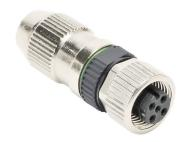
Murrelektronik field wireable connector, M12 nut 4-pin female axial connection, accepts cable diameter size 2.9-5.1mm, 22 - 26 AWG, insulation displacement (IDC) connection, IP67.
