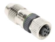
Murrelektronik connector, field-wireable, M12 nut 4-pin female axial connection, accepts cable diameter size 2.9-5.1mm, 22 - 26 AWG, insulation displacement (IDC) connection, IP67.
