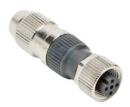
Murrelektronik connector, field-wireable, M12 nut 4-pin female axial connection, accepts cable diameter size 4-5.1mm, 20 - 24 AWG, insulation displacement (IDC) connection, IP67.
