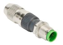
Murrelektronik connector, field-wireable, M12 barrel 4-pin male axial connection, accepts cable diameter size 4-5.1mm, 20 - 24 AWG, insulation displacement (IDC) connection, IP67.
