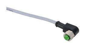
Murrelektronik connection cable, M12 right-angle female to pigtail, 5-pole, PVC jacket, gray, 32.8ft/10m cable length, IP67.
