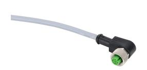
Murrelektronik connection cable, M12 right-angle female to pigtail, 5-pole, PVC jacket, gray, 9.8ft/3m cable length, IP67.
