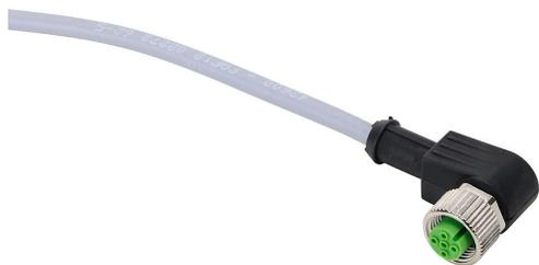
Murrelektronik connection cable, M12 right-angle female to pigtail, 4-pole, PVC jacket, gray, 49.2ft/15m cable length, IP67.
