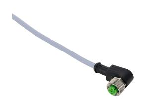
Murrelektronik connection cable, M12 right-angle female to pigtail, 4-pole, PVC jacket, gray, 32.8ft/10m cable length, IP67.
