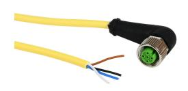
Murrelektronik connection cable, M12 right-angle female to pigtail, 4-pole, PUR jacket, yellow, 49.2ft/15m cable length, IP65 IP66K IP67.
