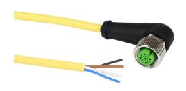
Murrelektronik connection cable, M12 right-angle female to pigtail, 4-pole, PUR jacket, yellow, 22.9ft/7m cable length, IP65 IP66K IP67.
