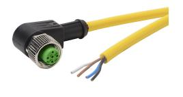
Murrelektronik connection cable, M12 right-angle female to pigtail, 4-pole, PUR/PVC jacket, yellow, 22.9ft/7m cable length, IP65 IP66K IP67.
