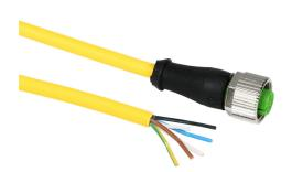
Murrelektronik connection cable, M12 axial female to pigtail, 5-pole, PUR jacket, yellow, 16.4ft/5m cable length, IP65 IP66K IP67.
