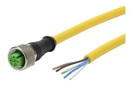
Murrelektronik connection cable, M12 axial female to pigtail, 5-pole, PUR/PVC jacket, yellow, 32.8ft/10m cable length, IP65 IP66K IP67.
