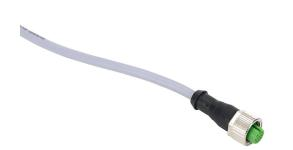
Murrelektronik connection cable, M12 axial female to pigtail, 4-pole, PVC jacket, gray, 49.2ft/15m cable length, IP67.
