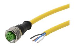
Murrelektronik connection cable, M12 axial female to pigtail, 4-pole, PUR/PVC jacket, yellow, 32.8ft/10m cable length, IP65 IP66K IP67.
