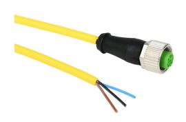
Murrelektronik connection cable, M12 axial female to pigtail, 3-pole, PUR jacket, yellow, 16.4ft/5m cable length, IP65 IP66K IP67.
