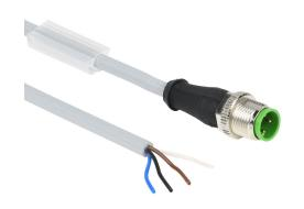
Murrelektronik connection cable, M12 axial male A-coded to pigtail, 4-pole, 250 VAC/VDC, 4A, 22 AWG, PVC jacket, gray, unshielded, 49.2ft/15m cable length, IP65 IP66K IP67, sensor & signal.
