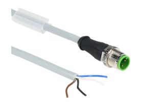
Murrelektronik connection cable, M12 axial male A-coded to pigtail, 4-pole, 250 VAC/VDC, 4A, 22 AWG, PVC jacket, gray, unshielded, 32.8ft/10m cable length, IP65 IP66K IP67, sensor & signal.
