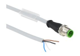
Murrelektronik connection cable, M12 axial male A-coded to pigtail, 4-pole, 250 VAC/VDC, 4A, 22 AWG, PVC jacket, gray, unshielded, 22.9ft/7m cable length, IP65 IP66K IP67, sensor & signal.
