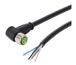
Murrelektronik connection cable, M8 right-angle female to pigtail, 5-pole, PUR jacket, black, 32.8ft/10m cable length, IP67.
