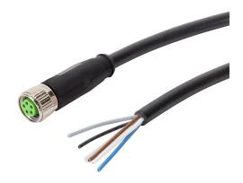
Murrelektronik connection cable, M8 axial female to pigtail, 5-pole, PUR jacket, black, 4.9ft/1.5m cable length, IP67.
