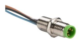
Murrelektronik bulkhead connector, M8 4-pin male to pigtail, 24 AWG, 1.6ft/0.5m cable length, nylon 12 conductor insulation material, IP67.
