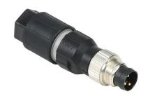
Murrelektronik connector, field-wireable, 3-pin M8 axial male A-coded, accepts cable diameter size 2.5-5mm, 24-20 AWG, insulation displacement (IDC) connection, IP65 IP67.
