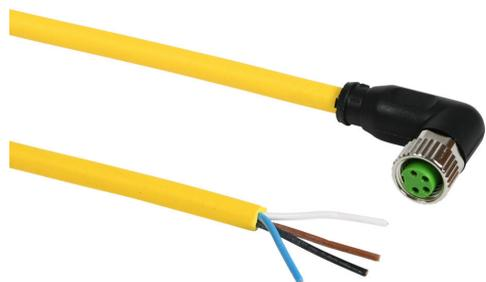
Murrelektronik connection cable, M8 right-angle female to pigtail, 4-pole, PUR jacket, yellow, 16.4ft/5m cable length, IP65 IP66K IP67.
