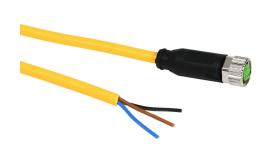
Murrelektronik connection cable, M8 axial female to pigtail, 3-pole, PUR jacket, yellow, 22.9ft/7m cable length, IP65 IP66K IP67.
