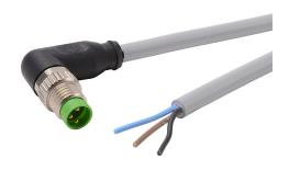
Murrelektronik connection cable, M8 right-angle male to pigtail, 3-pole, PVC jacket, gray, 16.4ft/5m cable length, IP65 IP66K IP67.
