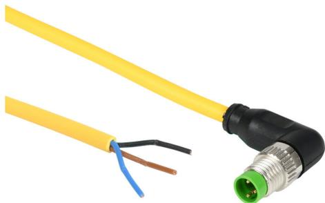
Murrelektronik connection cable, M8 right-angle male to pigtail, 3-pole, PUR jacket, yellow, 32.8ft/10m cable length, IP65 IP66K IP67.
