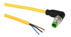
Murrelektronik connection cable, M8 right-angle male to pigtail, 3-pole, PUR jacket, yellow, 6.5ft/2m cable length, IP65 IP66K IP67.
