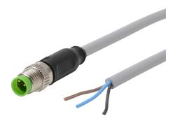
Murrelektronik connection cable, M8 axial male to pigtail, 3-pole, PVC jacket, gray, 32.8ft/10m cable length, IP65 IP66K IP67.
