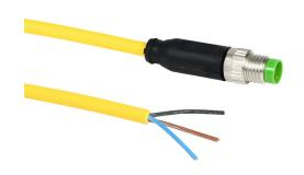
Murrelektronik connection cable, M8 axial male to pigtail, 3-pole, PUR jacket, yellow, 16.4ft/5m cable length, IP65 IP66K IP67.
