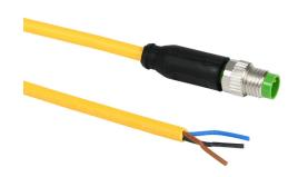
Murrelektronik connection cable, M8 axial male to pigtail, 3-pole, PUR jacket, yellow, 6.5ft/2m cable length, IP65 IP66K IP67.
