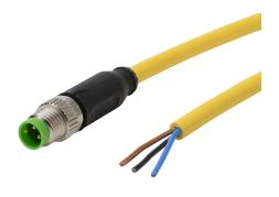
Murrelektronik connection cable, M8 axial male to pigtail, 3-pole, PUR/PVC jacket, yellow, 32.8ft/10m cable length, IP65 IP66K IP67.
