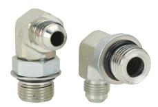
HY-TECH hydraulic fluid adapter, elbow, plated steel body, (1) -6 male JIC 37 deg and (1) -8 male o-ring boss. Package of 2.
