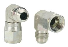
HY-TECH hydraulic fluid adapter, elbow, plated steel body, (1) -6 male JIC 37 deg and (1) -6 female JIC 37 deg. Package of 2.
