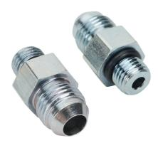
HY-TECH hydraulic fluid adapter, straight, plated steel body, (1) -6 male JIC 37 deg and (1) -4 male o-ring boss. Package of 2.
